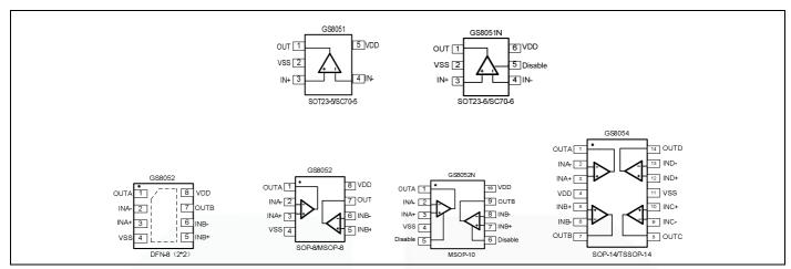
Figure 1. Pin Assignment Diagram
