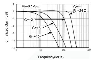
Inverting Small Signal Frequency Response
