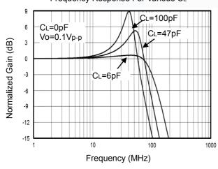
Frequency Response vs.Capacitive Load
