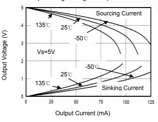
Output Voltage vs. Output Current
