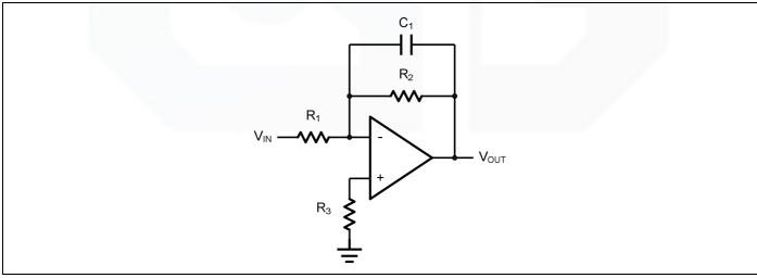
Figure 5. Low Pass Active Filter
